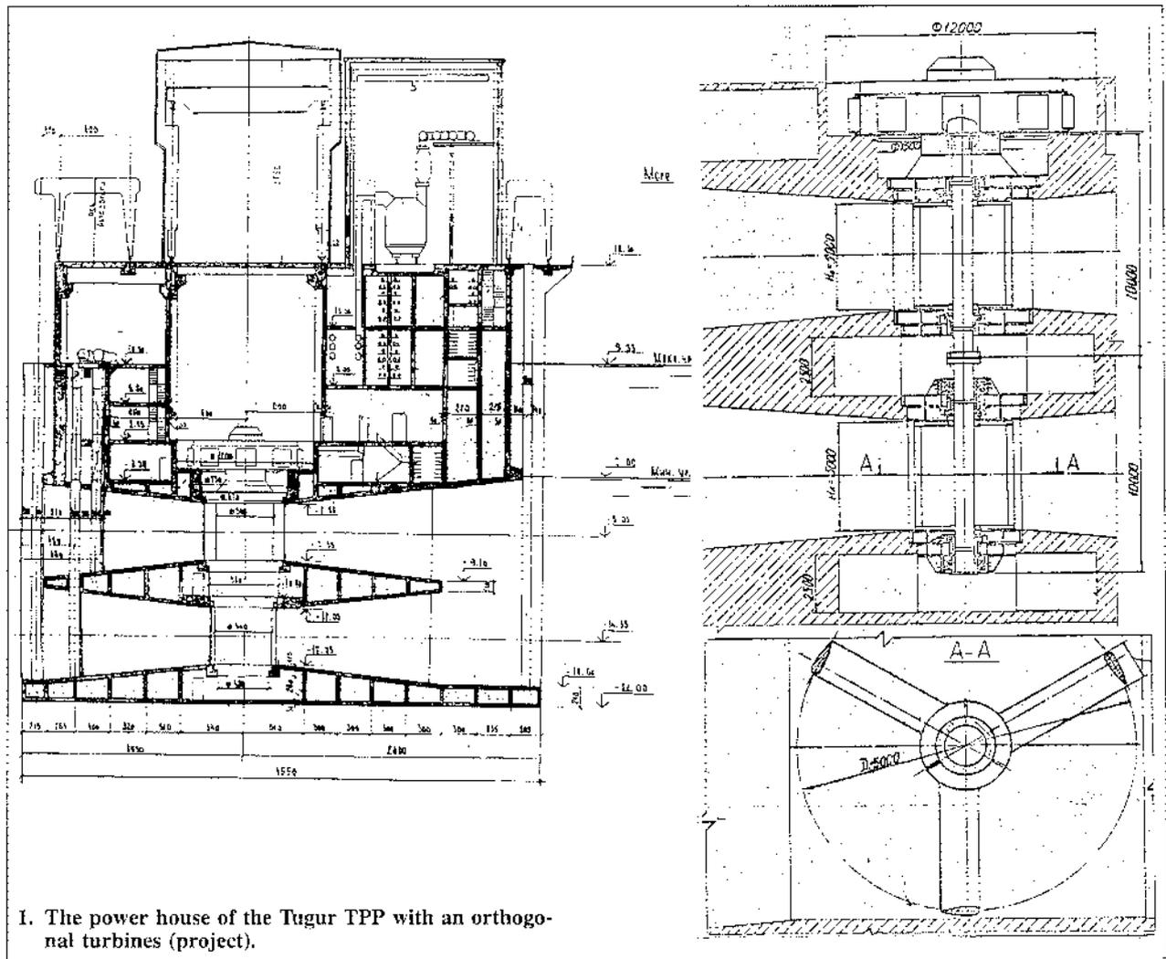
I. The power house of the Tugur TPP with an orthogonal turbines (project).
