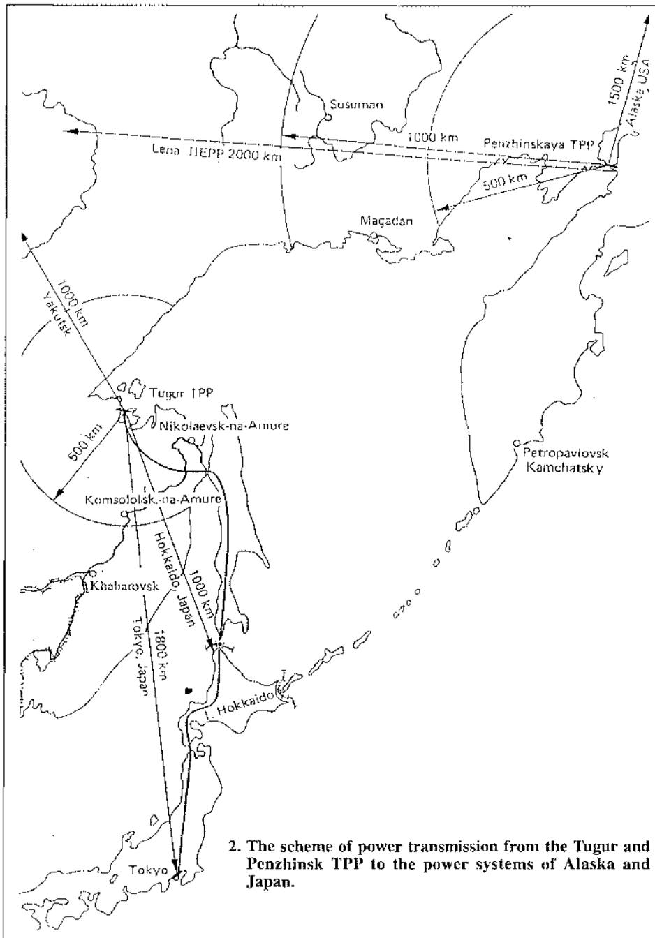
2. The scheme of power transmission from the Tugur and Penzhinsk TPP to the power systems of Alaska and Japan.
